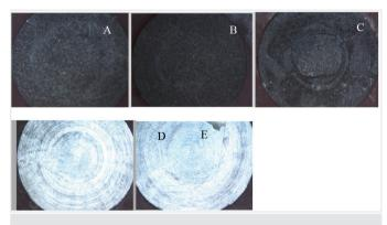
**Figure 2.** View of failure types; A- Adhesive type for sandblasted surfaces, B-Mixed type for sandblasted surfaces, C- Cohesive type for sandblasted surfaces, D- Adhesive type for non-treated surfaces, E- Mixed type for non-treated surfaces
